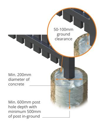
Important: For standard 50x50mm or 65x65mm aluminium posts, a fairly dry concrete mix can be used which will hold the post in place without any bracing while the concrete dries. However, the site must be revisited before the concrete sets firm to recheck post alignment. Any heavier posts, i.e. gate posts, should be concreted in place and braced until the concrete is dry.
